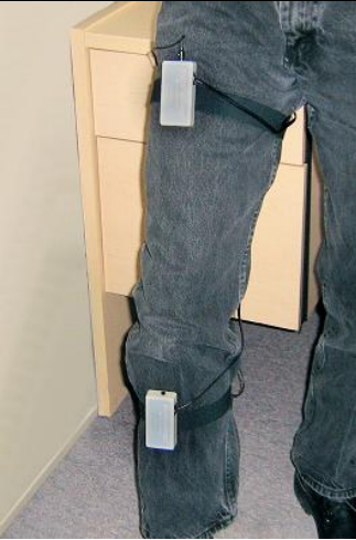
Position of the Inclinometer
